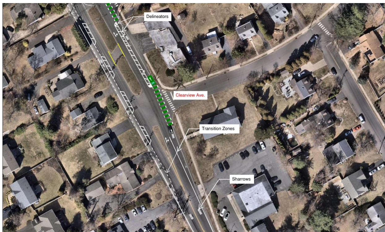
Figure 4 - Southern end of bike lanes showing delineators for motor vehicle right turns, transitions from shared lanes to bike lanes, and sharrows for shared lane use.
