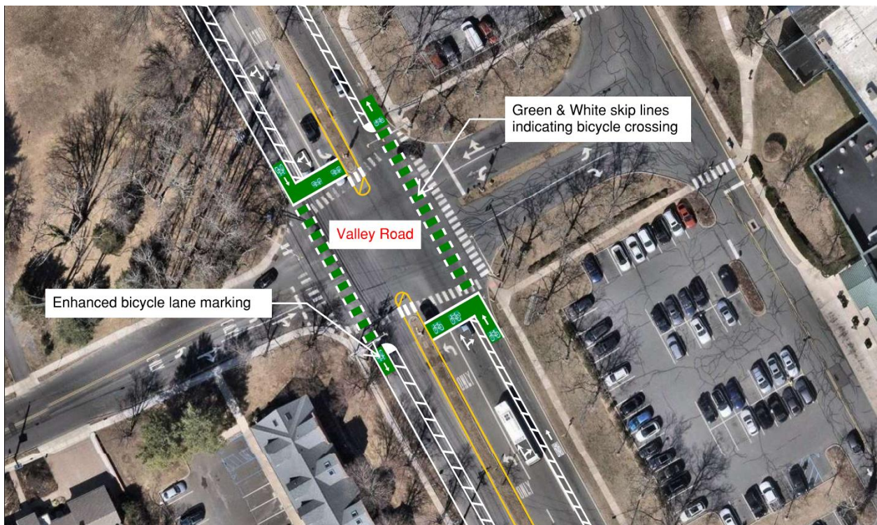
Figure 2 - Valley Road / PSC intersection showing green skip lines for bicycle crossing a major intersection and enhanced bike lane marking for motorist visibility
