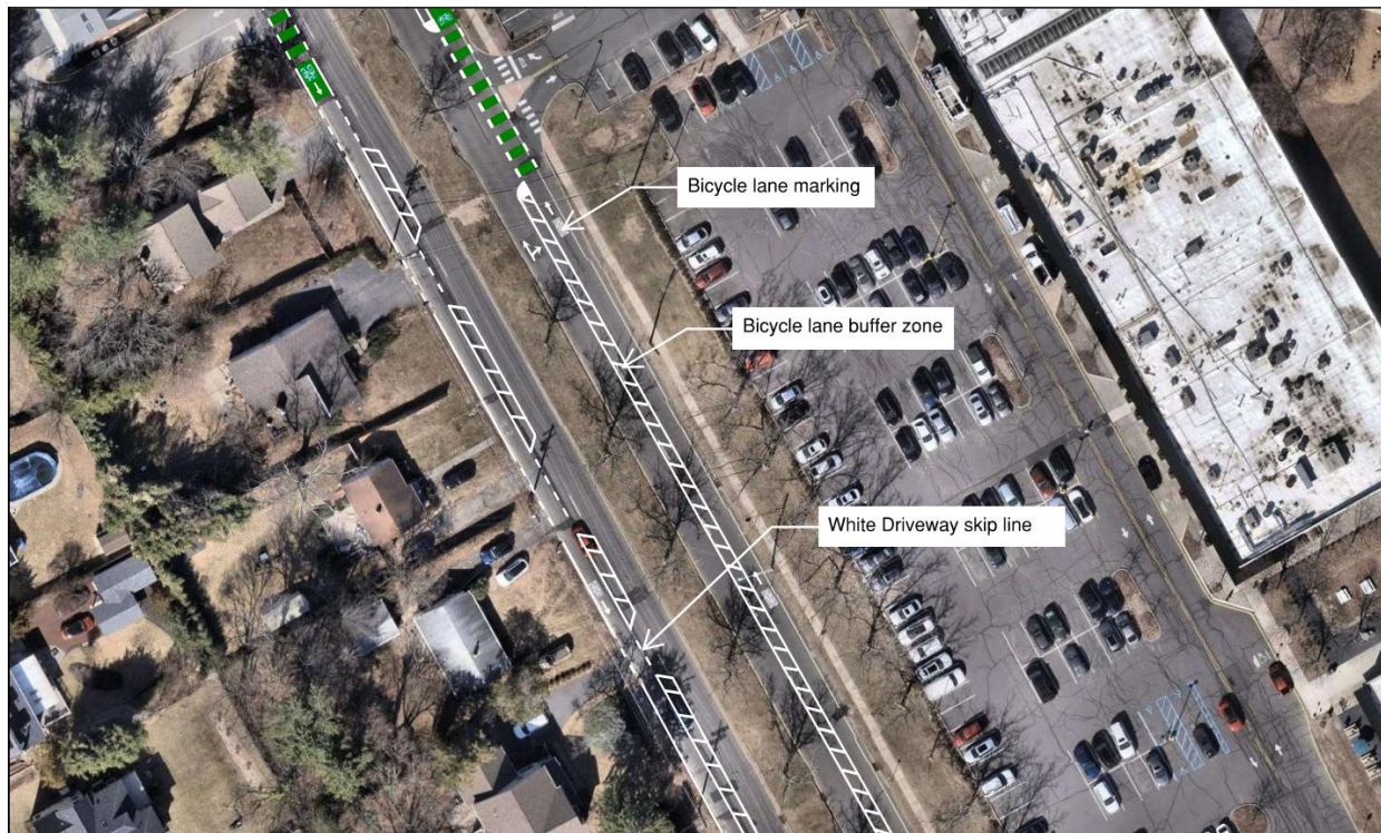
Figure 3 - Roadway section showing standard bike lane markings, buffer zone markings, and treatment at minor driveways
