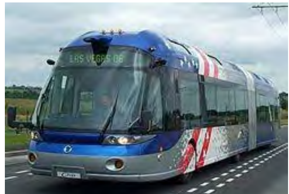
Figure 1-10 Civis optically guided bus operated by RTC in Las Vegas
