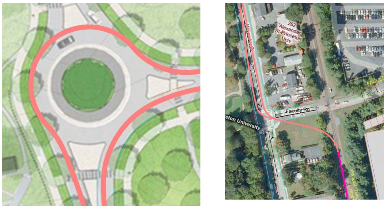
Figure 10: Streetcar alignment options through the Roundabout on left; on right, connection from Dinky line to Alexander Road in proximity of Faculty Road.
